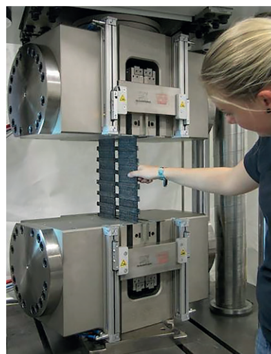
d) Example of hydraulic jaws for high-strength products
