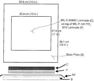
C = MIL-C-9084C Laminate, 20 nested plies of MIL-C-9084C Type 7781 glass cloth impregnated with test epoxy resin system
