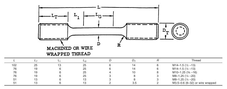
FIG. 2 Threaded Cylindrical Specimen (Dimensions in mm)
