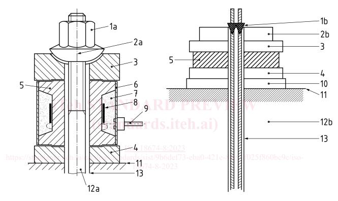
a) Spherical seat for a bar tendon
