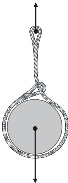
Figure 4 — Example of choker hitch
