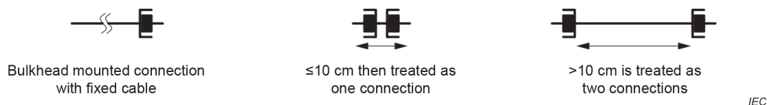
Figure 14 – Symbols for bulkhead connections
