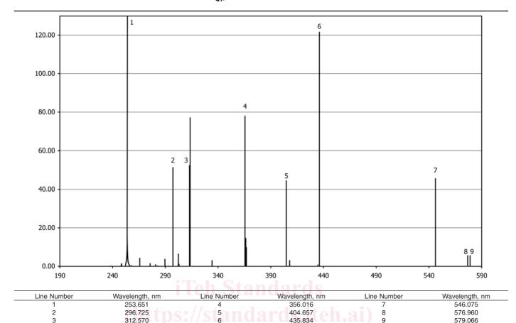
Instrument: Cary 5000 Scanning Speed: 1.2 nm/min Spectral Bandwidth: 0.05 nm Spectral Data Interval: 0.01 nm
