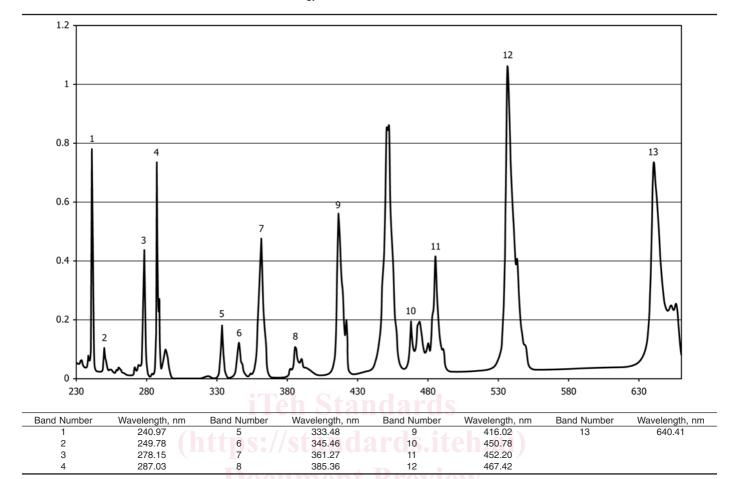
FIG. 3 Spectrum of 4 % Solution of Holmium Oxide in 1.4 M Perchloric Acid (1.00-cm Cell) Showing Reference Wavelengths (3)
