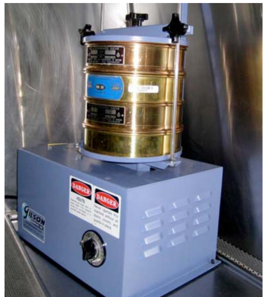
FIG. 1 Configuration of 20-cm Diameter Sieves on the Sieve Shaker
