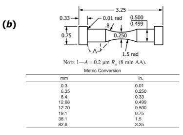
FIG. 1 Standard Hourglass Low Cycle Fatigue Specimen (Threaded Ends (a) and Button Head (b))
