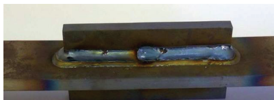
Figure 1 — Seam weld as 1-dimensional joint
