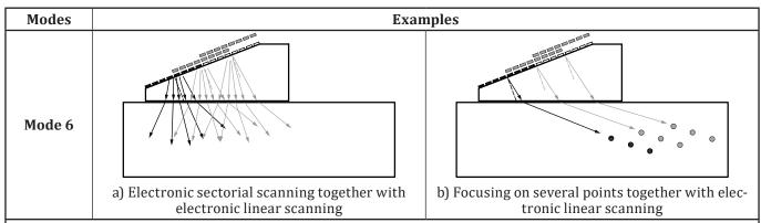
The medium between the array and the test object may be a fluid (immersion) or a solid (e.g. wedge).
