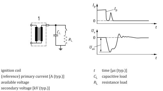
Figure 2 — Example of secondary voltage waveform
