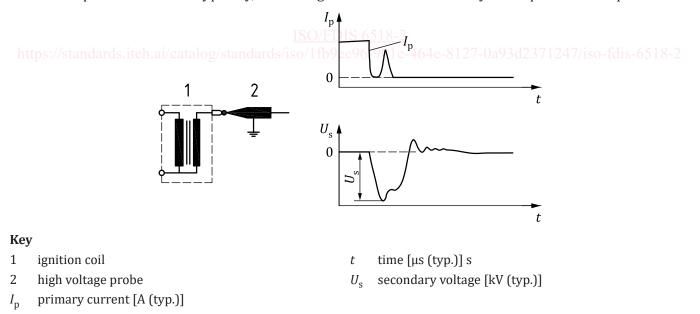
Figure 3 — Example of secondary voltage waveform
