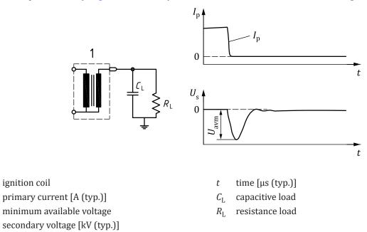
Figure 4 — Example of secondary voltage waveform for a fouled spark plug with a low shunt resistance
