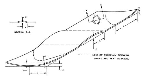
H = maximum distance between flat surface and lower surface of sheet. L = minimum distance between highest point on sheet and point of contact with flat surface. Flatness, percent =  $(H/L) \times 100$
