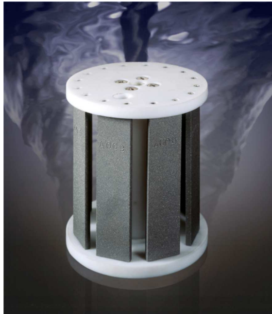
FIG. 2 Photo of Rotating Cage Containing Coupons—Gaps (Typically 0.85 \pm 0.01 cm) between the Coupons Introduce Localized Turbulence Coupons
