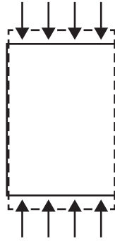
Figure 1 — Axial strain effects from the compressive effect of pressure
