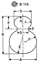
NOTE—For dimensions E, F and H the dimensional tolerance is ±0.016 in. (0.406 mm); for dimensions G and J the dimensional tolerance is ±0.008 in. (0.203 mm).
