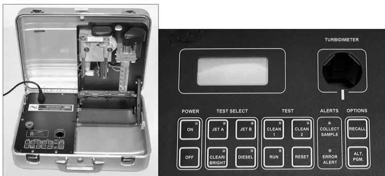
FIG. 2 Micro-Separometer Mark X and Control Panel
