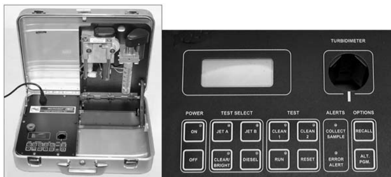
FIG. 2 Micro-Separometer Mark X and Control Panel
