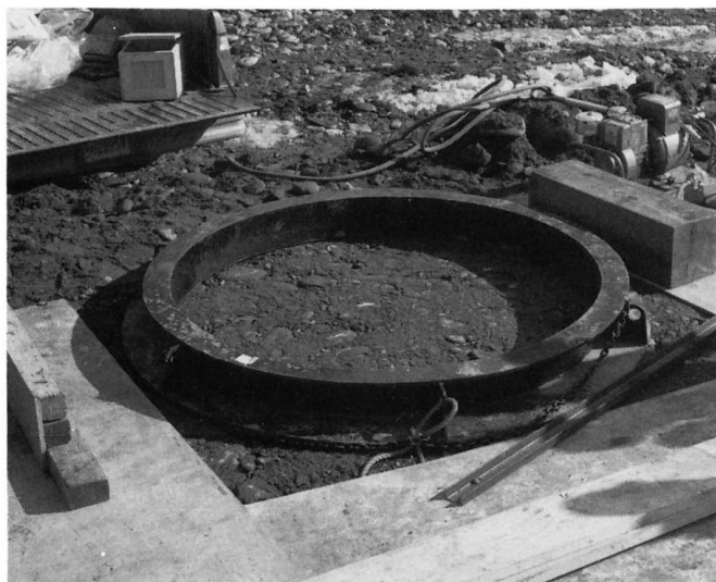
FIG. 1 A 6-ft ( 1.8-m )[1.8-m] Diameter Metal Ring for Determining In-Place Unit-WeightDensity
