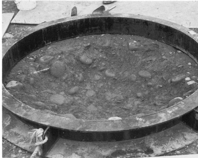
FIG. 4 Test Pit During Excavation
