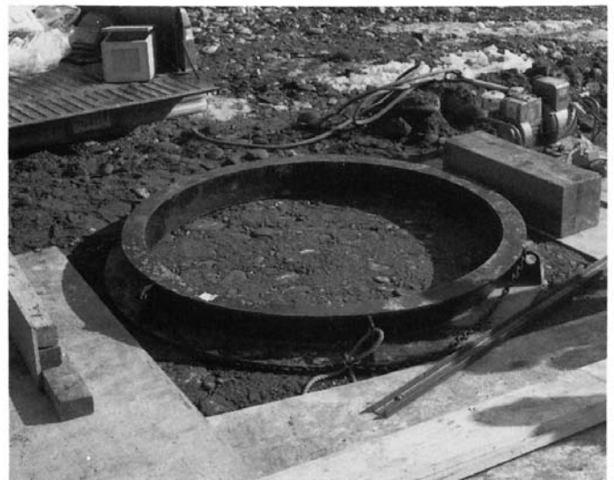
FIG. 1 A 6-ft [1.8-m] Diameter Metal Ring for Determining In-Place Density
