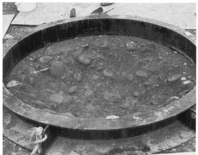
FIG. 4 Test Pit Excavation
