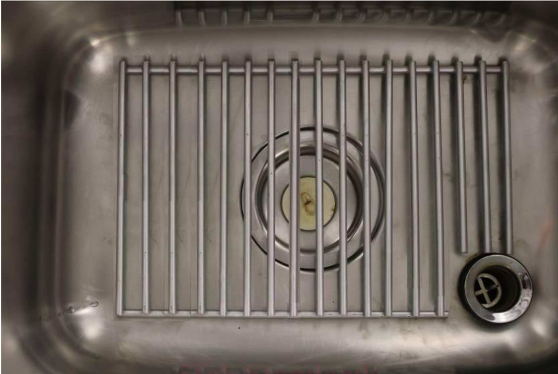
FIG. 4 Freezing Container with Tile Support Rack Installed
