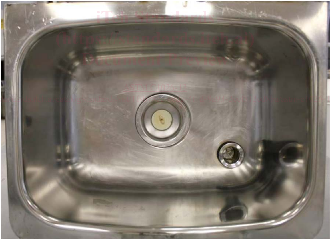
FIG. 3 Freezing Container Includes Low Point for the Thermocouple and Adjustable Overflow Drain in the Corner
