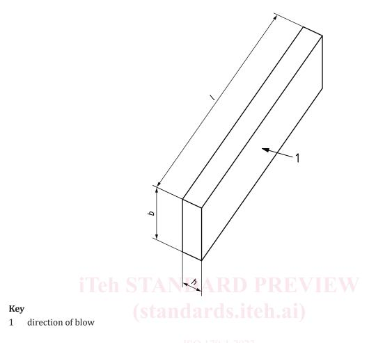
**Figure 3 — Charpy flatwise impact (f)** https://standards.iteh.ai/catalog/standards/file/172a05c/iso-179-1-2023
