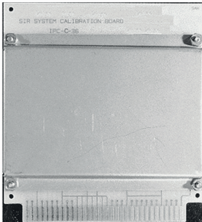
Figure 3 — Resistor verification board with protective cover
