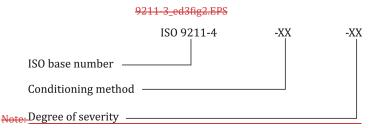
NOTE \_\_\_\_ The test code notation from ISO 9211-4 is slightly different in that this description does not include the statement "Coating environmental durability test". The coating environmental durability test name should be included as a descriptor to the environmental test code to avoid confusion, but is not directly a part of the environmental test code.
