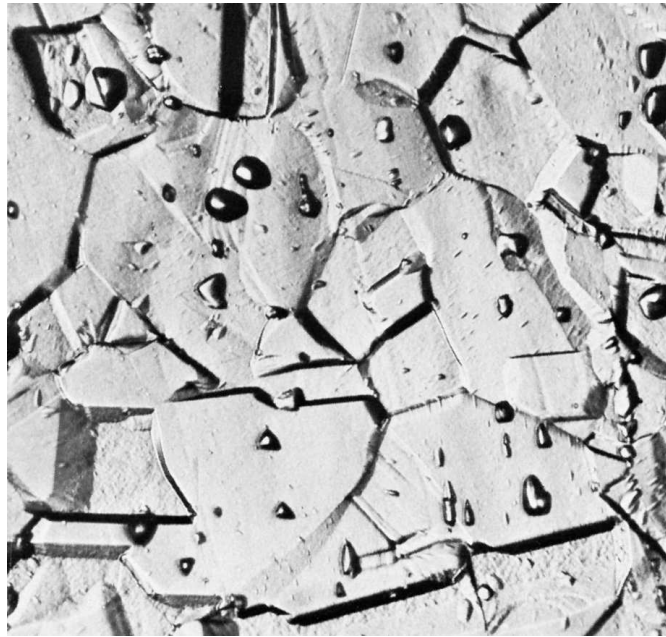
FIG. 1 Step Structure (500x) (Steps between grains, no ditches at grain boundaries)
