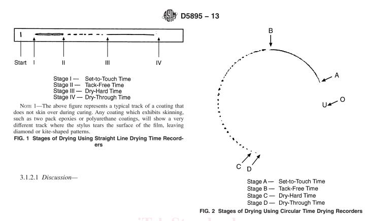
In these test methods, the dry-through time is reached when the stylus no longer left any visible mark on the film (see Fig. 1 and Fig. 2).
