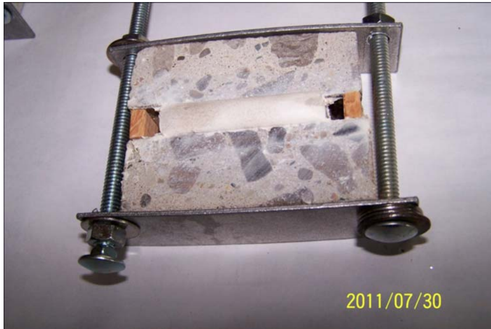
FIG. 3 Clamping Device Holding the Specimen in Compression
