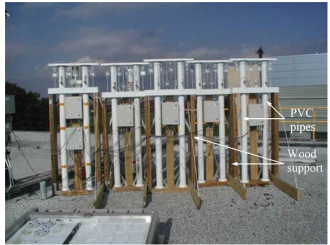
FIG. A1.2 Illustration of the Thermally Driven 'Winter/Compression' PVC Engine: A Global View
