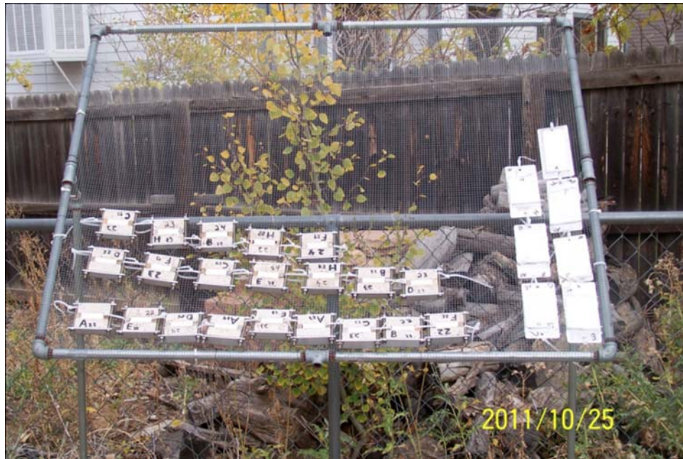
FIG. 5 Specimens Attached to Test Rack
