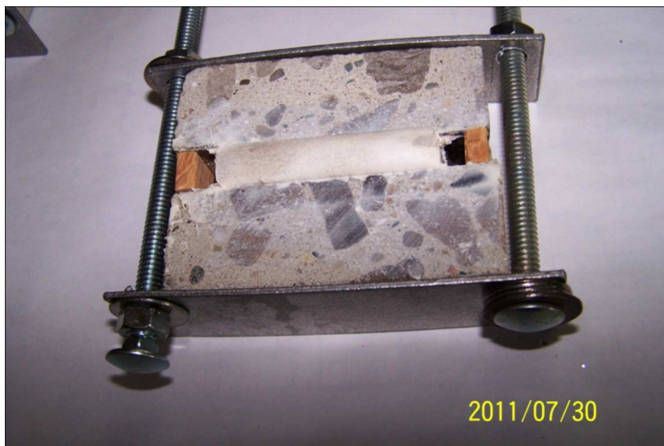
FIG. 3 Clamping Device Holding the Specimen in Compression
