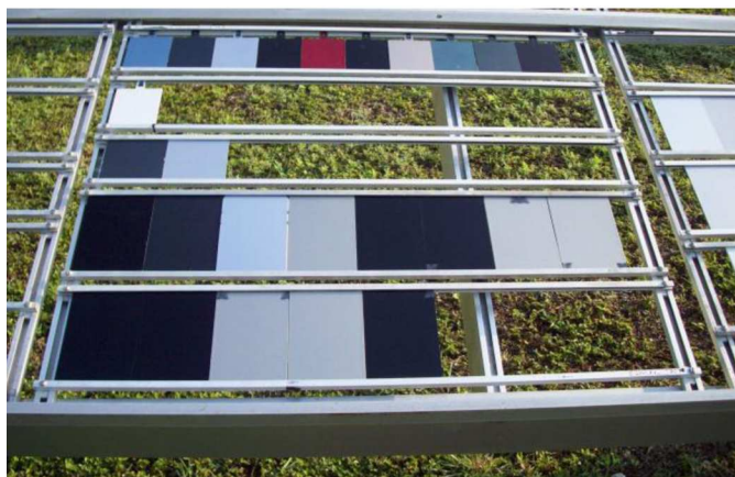
FIG. 1 Suitably Mounted Specimens in a Frame
