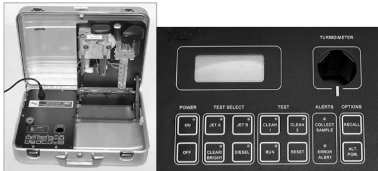
FIG. 2 Mark X Micro-Separometer and Control Panel
