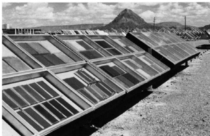
FIG. 2 Typical Non-Ventilated Enclosed Under Glass Exposure Cabinet, Type B (Black Box Under Glass)
