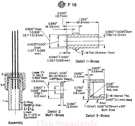
FIG. 1 Fixture for Making a Seal Between the Header Under Test and the Leak Detector
