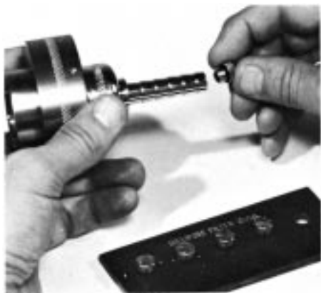
FIG. 3 Inserting a Typical Orifice
