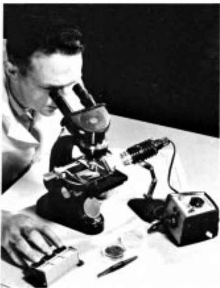
FIG. 1 Suitable Microscope: Inclined Binocular Body; Mechanical Stage; Triple Nosepiece; Ocular-Objective Combination to Obtain 40 to 45 \times and 90 to 150 \times Magnification
