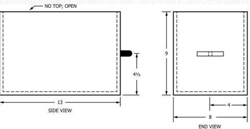
Note 1-Material specified is type 316 stainless steel (S.S.) or other suitable alloy (1/4 in. (6 mm) recommended).
