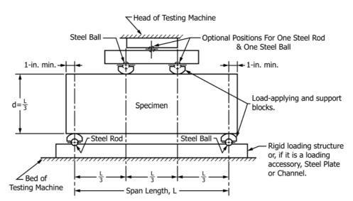
Note 1—This apparatus may be used inverted. If the testing machine applies a force through a spherically sealed head, the center pivot may be omitted, provided one load-applying block pivots on a rod and the other on a ball.
