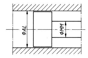
AL = cylinder boreMM = piston rod diameter
