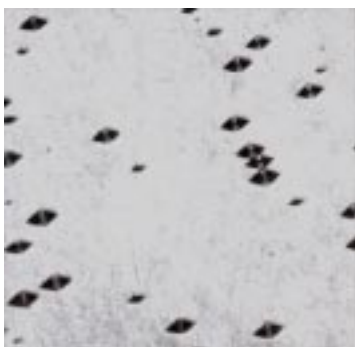
FIG. 2 Dislocation Etch Pits on (110) Silicon, Following 5-Min Wright Etch, Magnification 110×.
