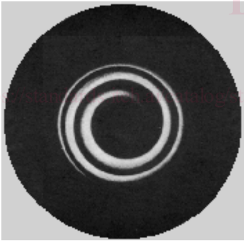
FIG. 26 Swirl Pattern Developed by Preferentially Etching a Czochralski Grown 10 to 20 ohm-cm Lapped Silicon Wafer.
