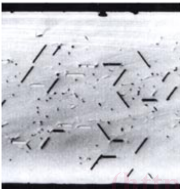
FIG. 19 Oxidation Induced Stacking Faults and Precipitates Found on the Cleavage Face of a Silicon Wafer After Thermal Treatment and 3-Min Secco Etch, Magnification 100 \times .
