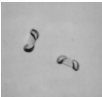
FIG. 12 Oxidation Induced Stacking Faults on (100) Silicon Following Oxidation and 4-min Wright Etch, Magnification 200X.
