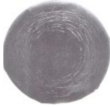
FIG. 27 A-swirl on as Grown Float-Zone Silicon Following Preferential Etch, Full Wafer View.
