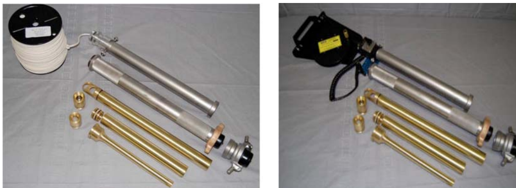
FIG. 4 Examples of Closed/Restricted Sampling Equipment
