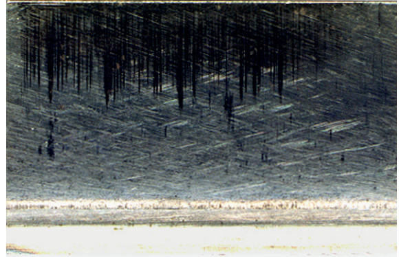
d) Approx. 15 mm failure marks
