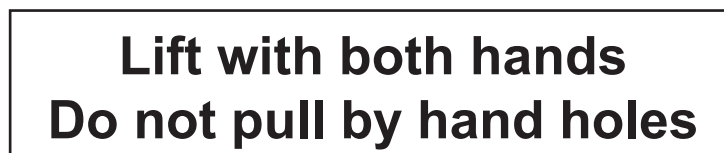
Figure 4 — Example of a caution sign for the correct use of hand holes
