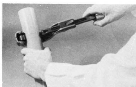
FIG. X3.1 Apparatus for Cutting Tube
