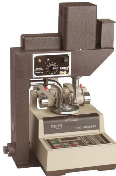
FIG. 1 Taber Abraser with Grit Feeder
