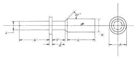
A = minimum expanded diameter of tubing as supplied.
