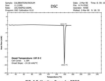
FIG. 2 Calibration Curve for PDSC
