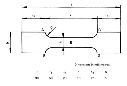
FIGURE - Shape and dimensions of test pieces
