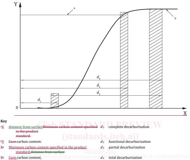
NOTE  $\div$  The depth of complete decarburization as described in  $d_1$  is determined by examination of the microstructure.
