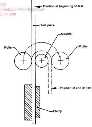
FIGURE 1 - Positions of clamp, mandrel and roller
