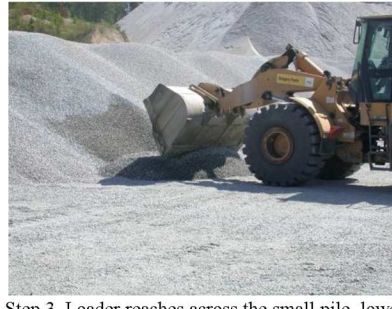
Step 3. Loader reaches across the small pile, lowers bucket, and back-drags small pile to form the sampling pad
