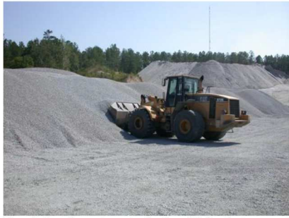
Step 1. Loader enters stockpile with bucket approximately 150mm [6 in.] above ground level
