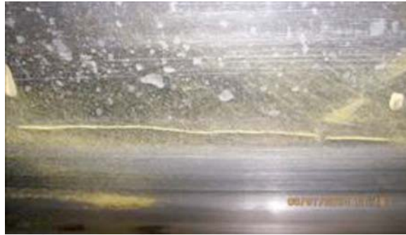
FIG. 3 Two cracks on a tooth just above the root that were only observed visually after being revealed by the ECA examination. In this example, the cracks were not apparent visually until MT was performed.
